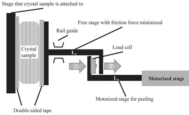
FIG. 1. Schematic of tensile testing machine used to measure the bonding energy between the layers of GaSeTe crystals.
