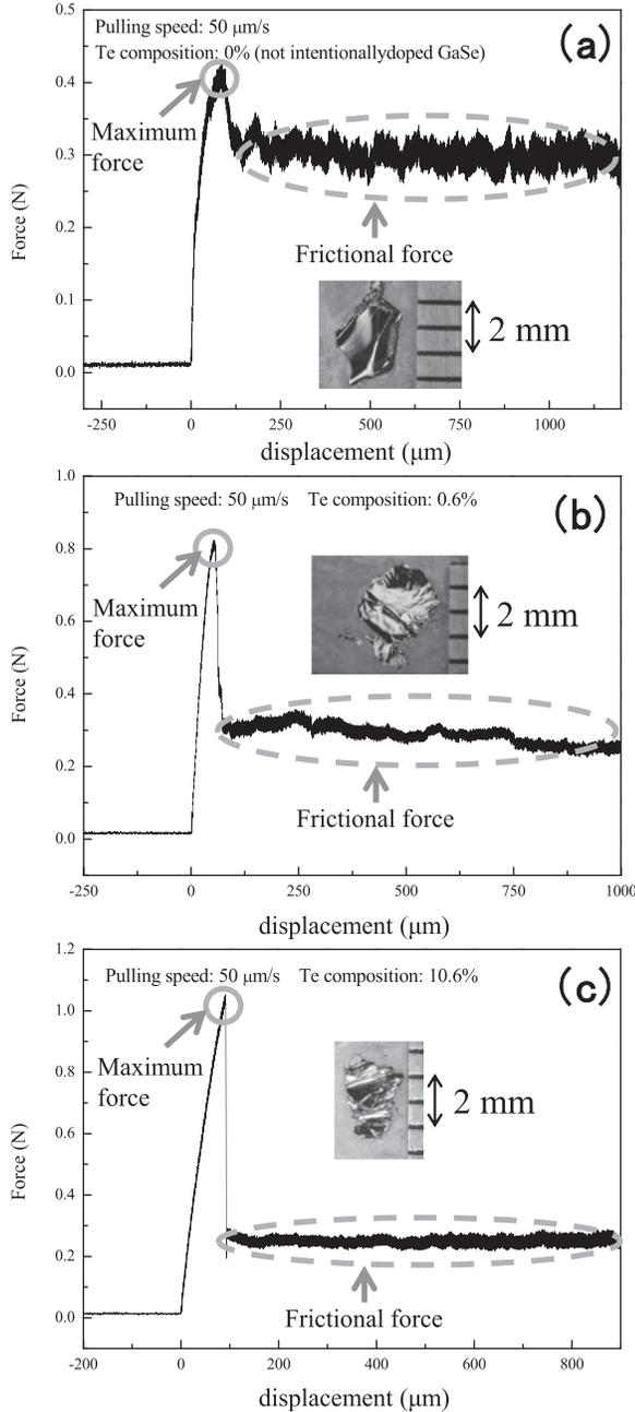
FIG. 2. Force measured by the strain gauge against the position of the slider,  $x$  ( $x=0$  denotes the contact position) for GaSe (a) and GaSe<sub>1-x</sub>Te<sub>x</sub> crystals with Te compositions of 0.006 (b) and 0.106 (c). Inset: photographs of the surfaces of the cleaved crystals.
